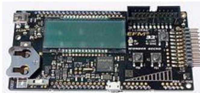
**Figure 6.** Energy Micro Wonder Gecko STK Board with EFM32WG990
